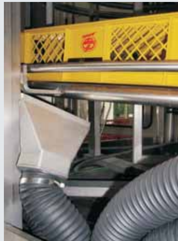
Lower blow-off nozzles
