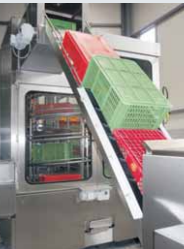
Slide from spiral washing zone to drying zone
