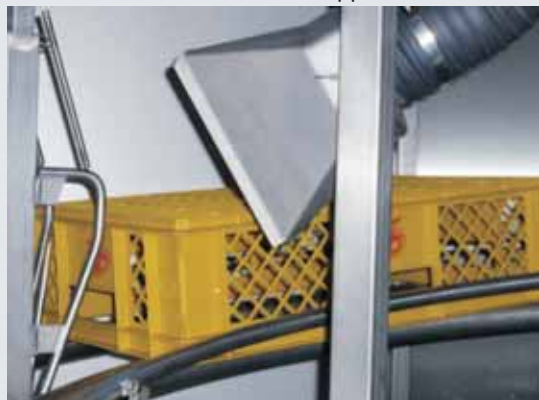
Upper blow-off nozzles
